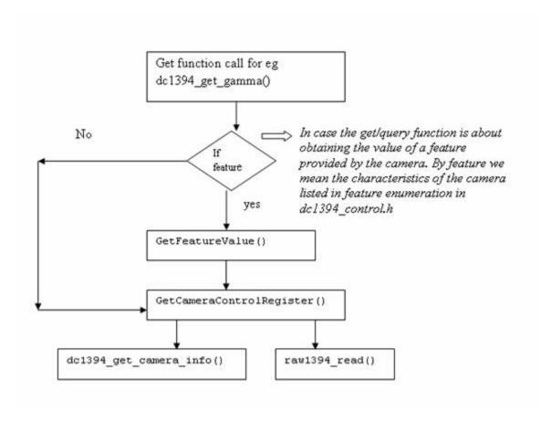
In case the get function you called is meant to retrieve the value of a camera feature (the value for the parameters listed in feature enumeration), that get function will call another get function (GetFea-
