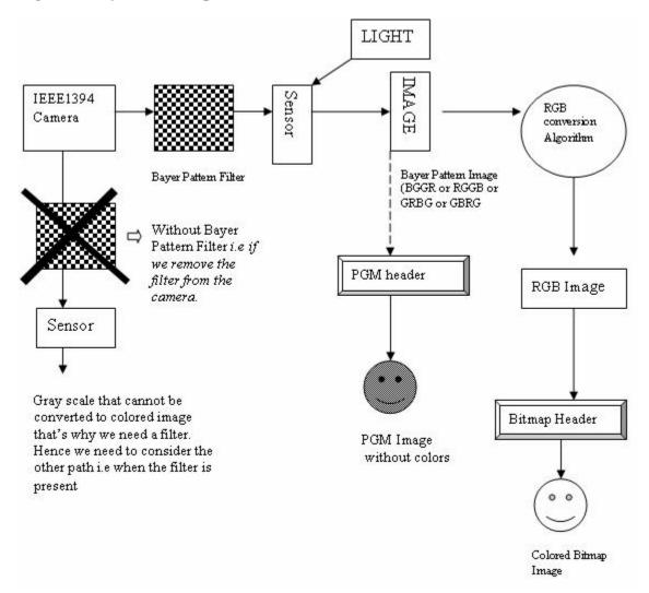
Let's understand how the RAW to RGB conversion algorithms work. We will look into the Nearest Neighbor algorithm in detail. Other Algorithms are thoroughly explained at the following web link: http://www-ise.stanford.edu/~tingchen/main.htm.
