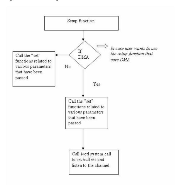
As shown in Figure 3, the Setup function in turn calls various set functions to set the parameter values to the camera registers. In the case of DMA setup, after the set functions have been called the ioctl system call is called to allocate memory for the DMA buffers and returns a pointer capture\_buffer in user space.
