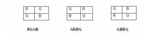
The image we obtained in the previous example was a Bayer Pattern image also known as a *RAW* image. This was stored in camera.capture\_buffer. In order to view what we have captured we convert this RAW image to .PGM by adding a header (look at the explanation in the section called "Example: How to grab image from the IEEE1394 camera").
