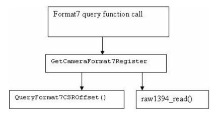
The Format7 query function will call GetCameraFormat7Register, which is supposed to read the values from the control and status registers of the camera. This function in turn will call the QueryFormat and CSROffset to know the offset for the particular information that has been queried. After getting the offset, raw1394\_read is used to actually read the values.
