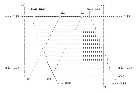
This is a generic monitor mode diagram. The x axis of the diagram shows the clock rate (DCF), the y axis represents the refresh rate (RR). The filled region of the diagram describes the monitor's capabilities: every point within this region is a possible video mode.
